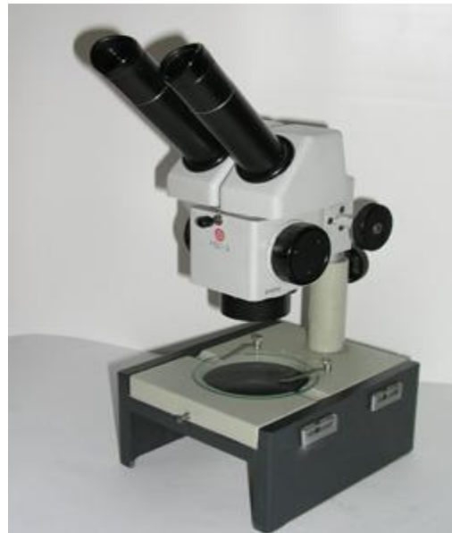
Fig. 1. Optic magnifying apparatus: A – Hand magnifying glass; B – Stereomicroscope MBC - 10
