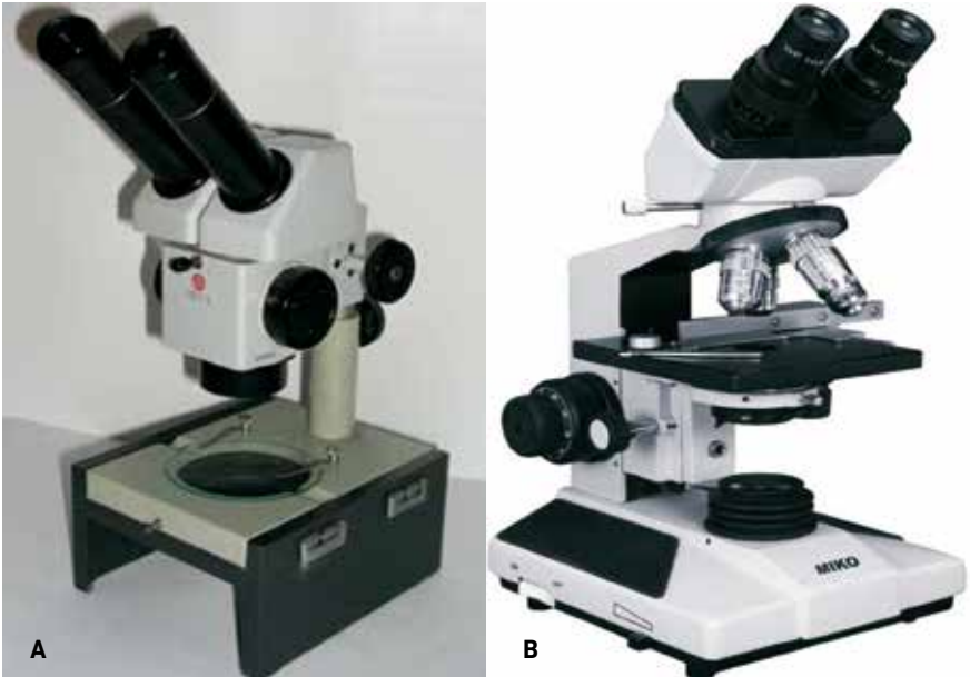
Fig. 2. Microscopice optice: A – stereomicroscop MBC-10; B – microscop optic (fotonic) Miko.
